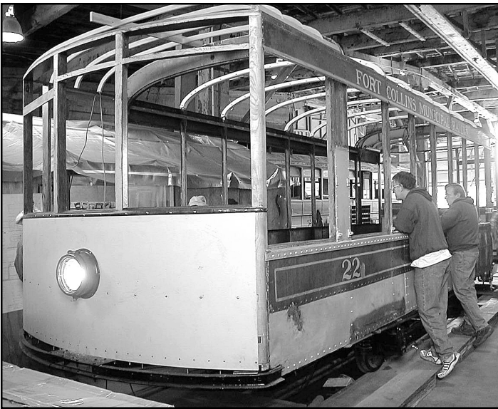
Rocky Mountain Railroad Club's Birney Car #22 on loan to the Pikes Peak Historical Street Railway Foundation as it looked on October 20, 2001. New steel ends and the roof ribs are starting to go into place. – Two photos © Thomas Peyton
