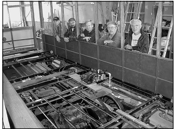
A view of all the new pipe work that has gone into the Birney's under carriage. Smiling proudly are Grant Harrison, Patrick Ayers, Gary Harrison, Vince Morris, and Jeff Smith. These workers are the main volunteers working on car #22. They are proud of the work that they have already put into the car.
